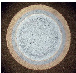
Ball Crater Test 100x magnification
